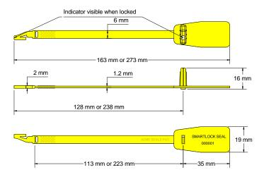
The Acme **Smartlock Seal** is a fixed length seal manufactured from Polypropylene material. The design features a strong single point locking mechanism and an indicator which protrudes through a hole in the underside of the locking head signifying it has been correctly locked. The seal also features a break off point for easy removal making this seal suitable for most applications.
